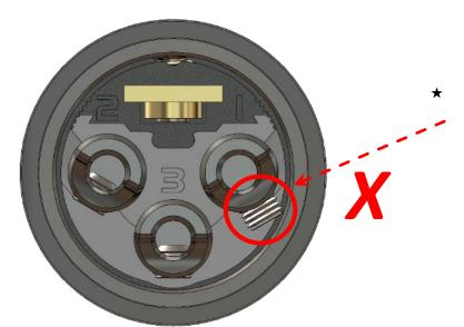
When using M2.5 \* 2 mm the hexagon socket set screw fixed conductor wire, the screw should not protrude from the screw hole and make contact with the connector housing – this could cause a s short circuit.
