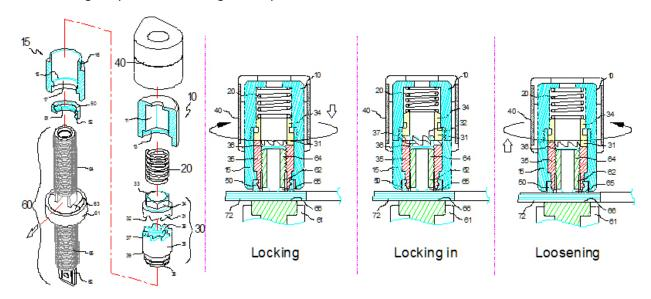
20 = Preset torsion spring • 30 = Ratchet-screws down until torsion spring prevents further tightening 40 = Polycarbonate housing adjusts settings between 10, 15, 30 and 50 • 60 = Main conductor 62/63 = one-piece pure-copper construction • 64/65 = POM plastic injection molding improves damping
